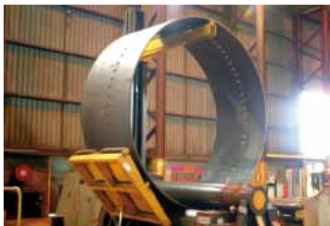
Wind Mill Tower Production Lines guaranteeing highest productivity rates and superior rolling quality (no-rerolling)
